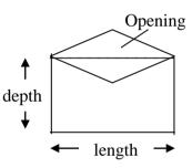
Over 100 mm in depth - opening not over 115 mm in length
