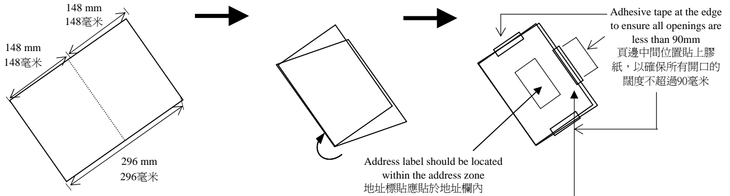
Figure 2 : Folder of A4 (296mm) size with 2 folds 圖示二：兩摺的A4(296毫米)尺寸紙張
